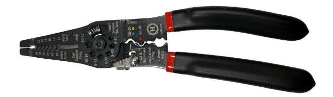
Very high quality multi-purpose stripper (20 - 10 AWG), insulated and non-insulated crimper (22 - 12 AWG), bolt cutter (4 - 40, 5 - 40, 6 - 32, 8 - 32, 10 - 32, 10 - 24) and wire cutter. Comfortable cushion grips.
